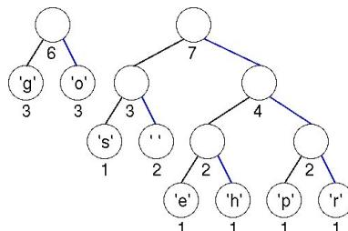
Finally, the last two trees are joined into a final tree whose weight is 13, the sum of the two weights 6 and 7. This tree is the tree we used to illustrate Huffman coding
